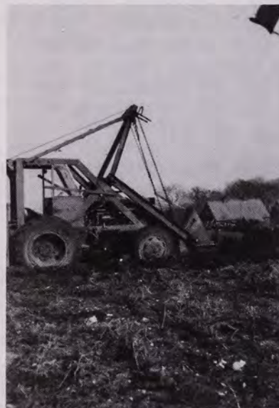
"Another early refinement was a Chaseside mechanical loading shovel..."
