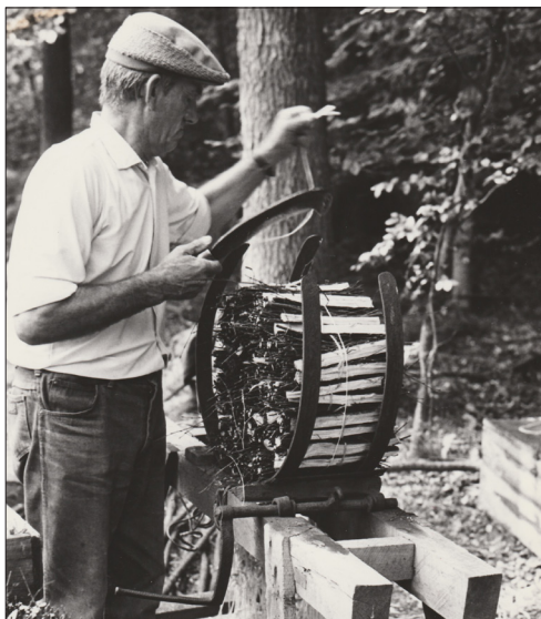
7 The firmly tied pimps are placed within the pimp machine.
