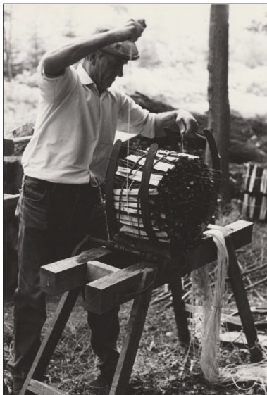
9 Once pressed, the pimps can be tied together as a single bundle.
