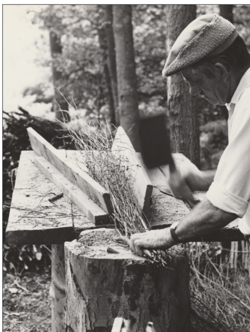
2 An already prepared birch faggot laid out on the 'boy' is cut to the desired length of ten inches.
