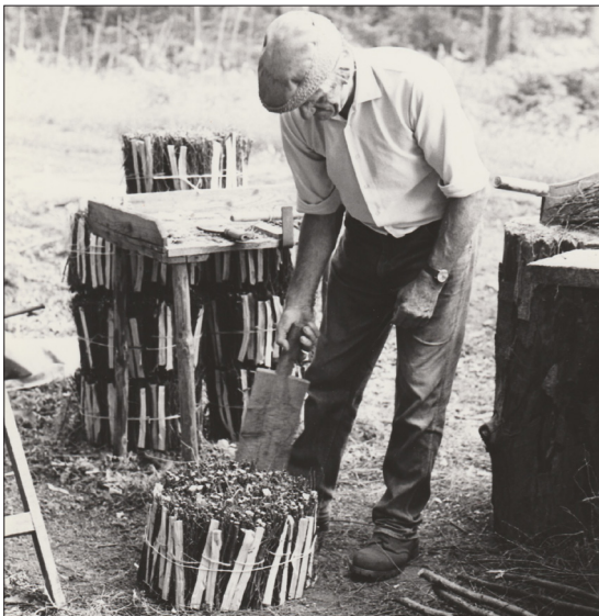
10 Released from the frame, a short-handled bat or paddle is used to pat the brushwood down to make a neat finish.
