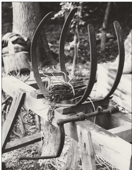
6 A strap attached to a handle mechanism compresses the bundles together inside a circular iron frame called a pimp machine.
