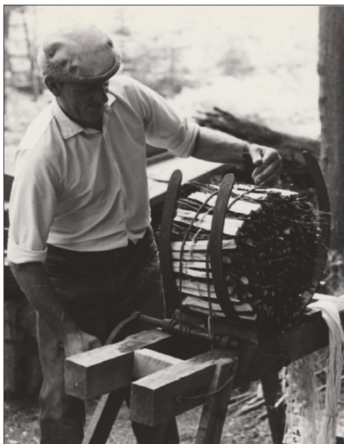
8 The pimp machine when filled holds 25 pimps.
